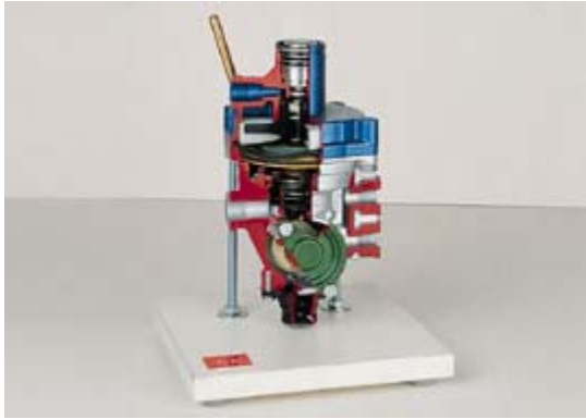
Order no. 1109 Automatic load-dependent brake power distributor
