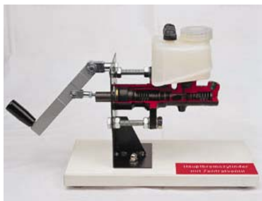
Order no. 1068 Graduated Tandem main brake cylinder with central valve
