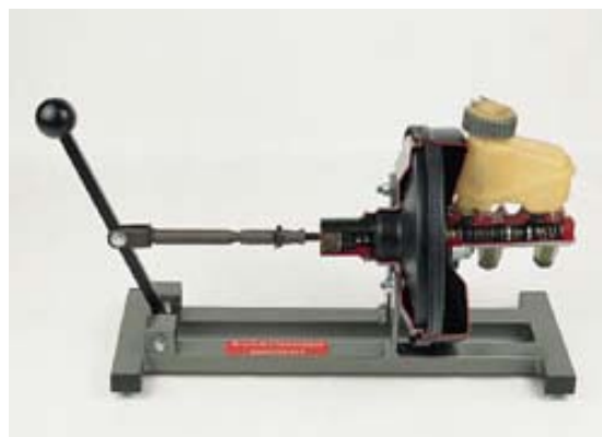
Order no. 1236 Pneumatic brake power assist unit with tandem brake master cylinder
